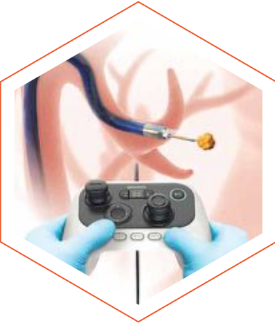
The Monarch Platform allows doctors to use an innovative telescoping design to navigate through the lungs with greater reach, vision and control.
